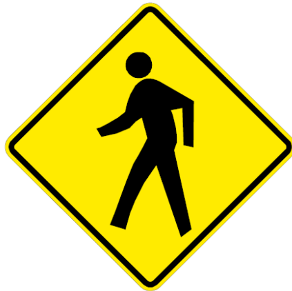
Figure A6. Advance Warning Sign
